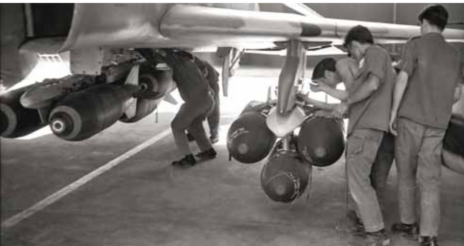
The M117 was used by the IDF/AF in two variants: the M117 MAU-91 high drag tail with standard fins and the MAU-103A low drag tail featuring conical fins with strakes. Although the weapon had a nominal weight of 750 lb (343 kg), its actual weight, depending on fuse and retardation options, is around 820 lb (373 kg). The bomb, however, lacked the force and precision to destroy hardened or heavier targets such as bridge struts or small bunkers, thus it was to be phased-out during the mid 1980s.
