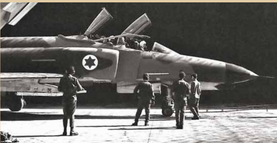
Photographed after YKW, Karpada #322 (Nickle Grass F-4E Block 37 USAF 68-0333) still features the early production block 'hardwing' configuration without manoeuvring slats. Of interest is the artwork on the gun cover just aft of the muzzle, applied when the aircraft belonged to the 33rd TFW. Note the suspensions for the AGM-45 'Shrike' anti radiation missile (ARM) on both inner wing pylons.
