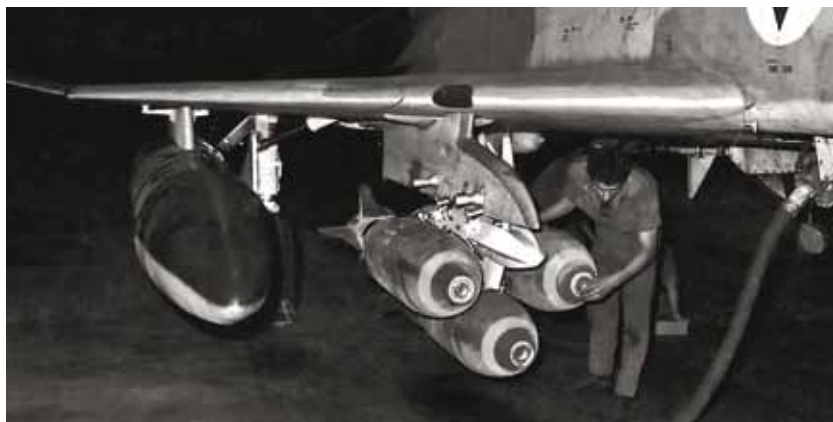
During the first weeks of the War of Attrition ground crews were able to gain substantial experience in arming and unarming their aircraft. In the top picture M117 bombs receive their fuses shortly prior to a bombing mission, while in the photograph below four airmen load a 90 kg heavy AIM-9D, IAF code Dekker (Rapier), on the left inboard pylon of a Kurnass.
